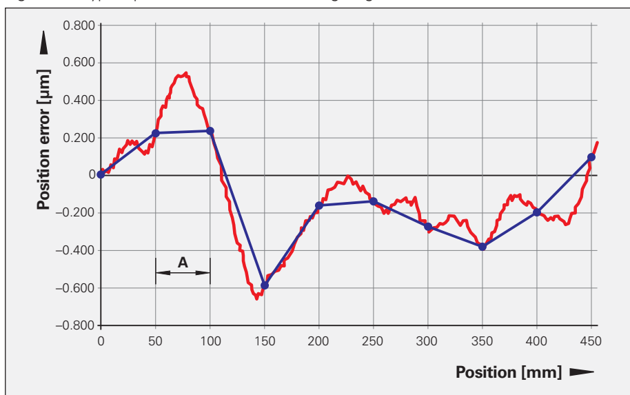
Figure 2: Compensation points for multipoint linear error compensation
