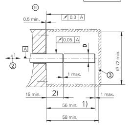
Tolerancing ISO 8015 ISO 2768:1989-mH ≤ 6 mm: ±0.2 mm
