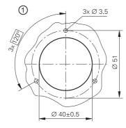
mm Tolerancing ISO 8015 ISO 2768:1989-mH ≤ 6 mm: ±0.2 mm
