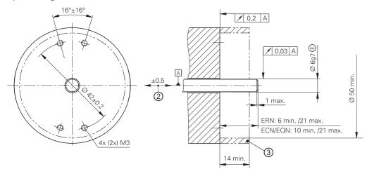
Tolerancing ISO 8015 ISO 2768:1989-mH ≤ 6 mm: ±0.2 mm
