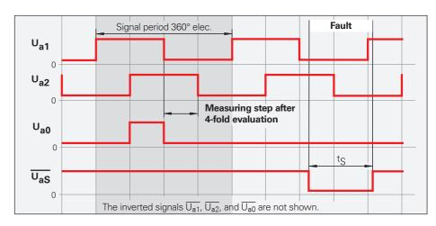
The distance between two successive edges of the incremental signals  $U_{a1}$  and  $U_{a2}$  through 1-fold, 2-fold, or 4-fold evaluation is one **measuring step**.
