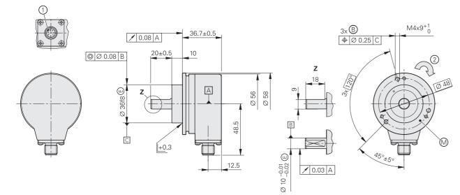
Tolerancing ISO 8015 ISO 2768:1989-mH ≤ 6 mm: ±0.2 mm
