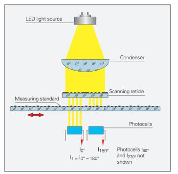
Photoelectric scanning in accordance with the imaging scanning principle
