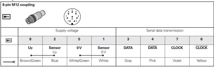
Cable shield connected to housing; U<sub>P</sub> = Power supply voltage Sensor: The sense line is connected in the encoder with the corresponding power line.
