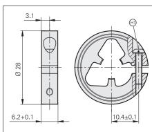
③ = X8 clamping screw with hexalobular socket; tightening torque: 1.1 Nm ±0.1 Nm
