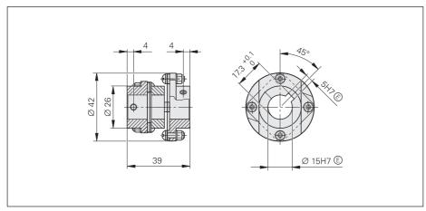
Tolerancing ISO 8015 ISO 2768:1989-mH ≤ 6 mm: ±0.2 mm
