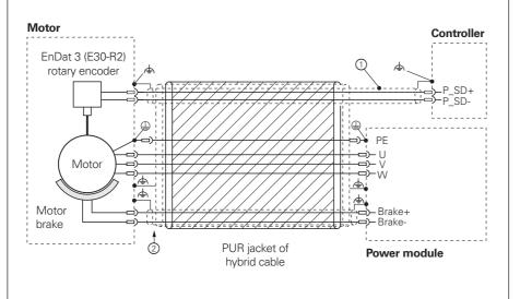
1 = Accidental contact of the shield with other metal parts must be prevented 2 = Shields connected to the housing on the connector side
